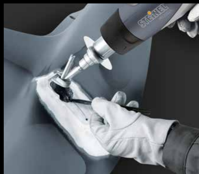
Repairing crack in bumpers.
