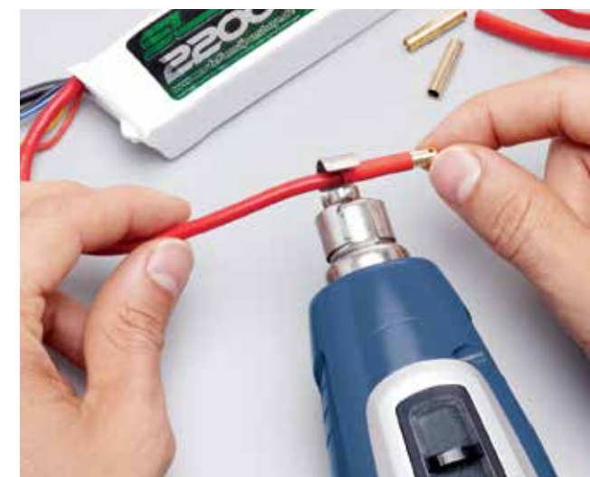
Heat-shrinking. Secure standing for hands-free work.
